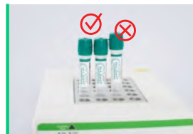
Fully insert the test tubes inside the wells of the incubator Incubate the samples for 24 hours [+/- 1 hour]
