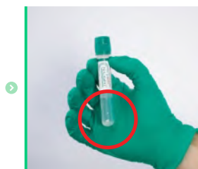
Verify the tablet is released into the liquid Start a timer (10min)
