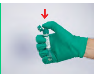
Hold the tube vertically Open the lid and firmly push the button to release the AquaSpark™ tablet
