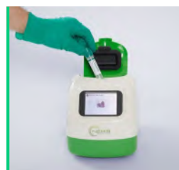
Place the test tube into the luminometer Start the measurement
