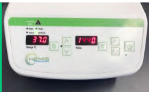
Set the temperature to 37°C and press <on> Set a timer for 24 hours [+/- 1]
