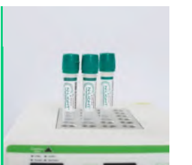
Put activated tubes back at 37°C Shake tubes again after 5 minutes to ensure good distribution of AquaSpark™
