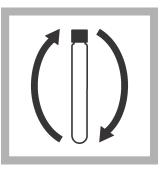
**3.** Put the cap on the vial. Invert to mix.
