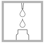
**4. Prepare the sample:** Add 5.0 mL of sample to a second Reactive High Range Phosphorus Test 'N Tube Vial.
