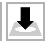
**11.** Insert the vial into the 16-mm cell holder.
