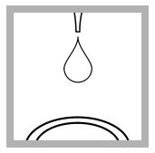
**9.** Add 1 drop of ECR Masking Reagent Solution into a clean square sample cell.
