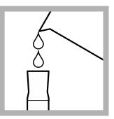
**2. Prepare the sample:** Fill a mixing cylinder to the 20-mL line with sample.
