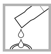
**11.** Pour 10 mL of the solution from the mixing cylinder into the sample cell.
