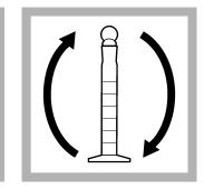
**4.** Put the stopper on the mixing cylinder. Invert the mixing cylinder several times to fully dissolve the powder.
