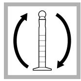
7. Put the stopper on the mixing cylinder. Invert the mixing cylinder several times to mix. The solution color becomes
