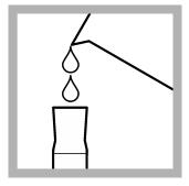
**4.** Rinse a clean 50-mL plastic graduated cylinder with the sample three times.
