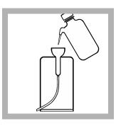
**15.** Immediately after use, flush the Pour-Thru Cell with at least 50 mL of deionized water.
