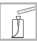
**11.** When the timer expires, pour the contents of the graduated cylinder with the blank sample into the Pour-Thru Cell.
