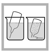
3. Tap the bottom of a NitraVer 5 Nitrate AccuVac Ampul to dislodge the powder. Fill the Ampul with sample. Keep the tip immersed while the Ampul fills completely.
