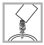
**3.** Add the contents of one NitraVer 5 Nitrate Reagent Powder Pillow. Put the stopper on the sample cell.
