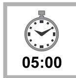
**6.** Start the instrument timer. A 5-minute reaction time starts. Keep the sample still while the timer counts down. An amber color shows if nitrate
