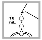
2. Prepare the blank: Fill a sample cell with 10 mL of deionized water.
